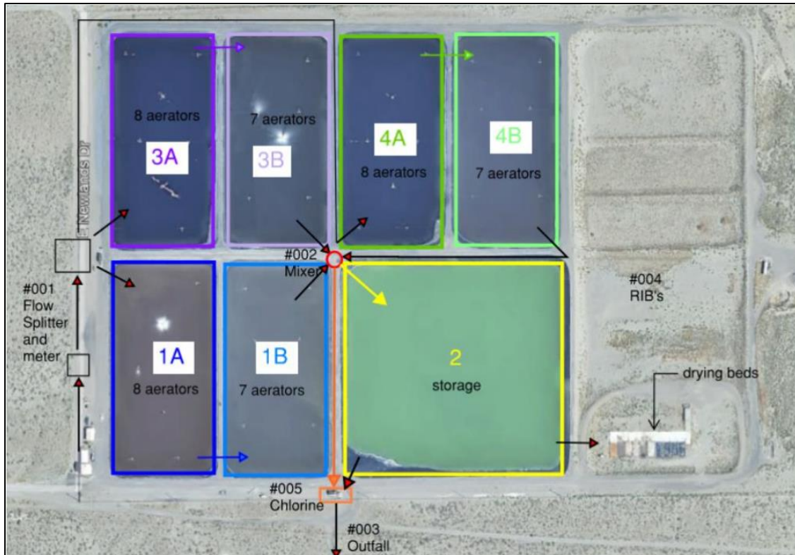
Figure Error! No text of specified style in document.-1 City of Fernley EWWTP showing Ponds 4A & 4B to be relined.
