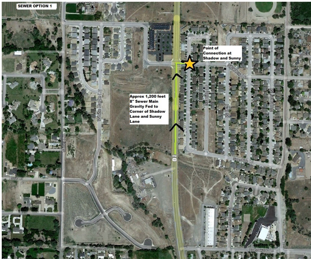
Figure 1 – Recommended Path of Extension of 8" Sewer Main
