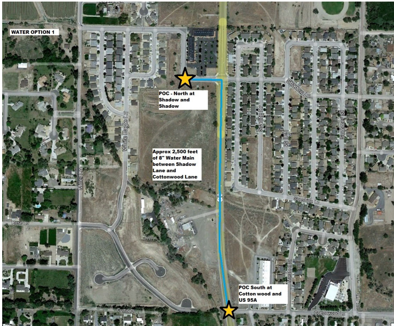
Figure 2 – Recommended Path of Extension of 8" Water Main
