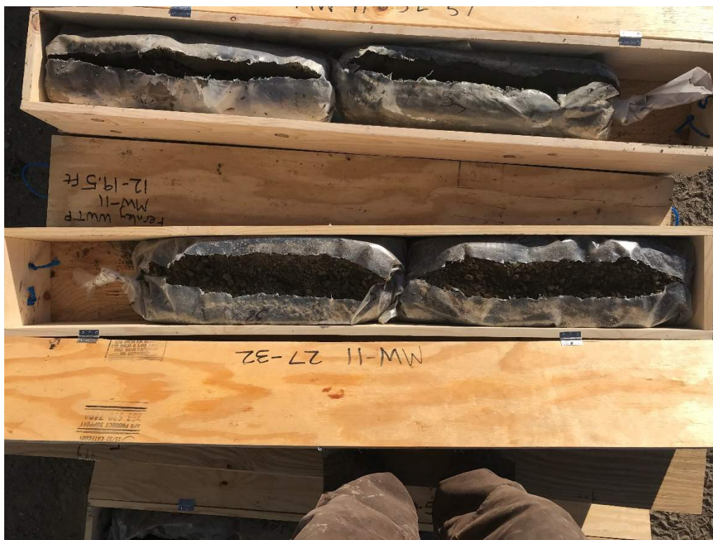
Figure 8. Sonic drill core in wooden storage boxes
