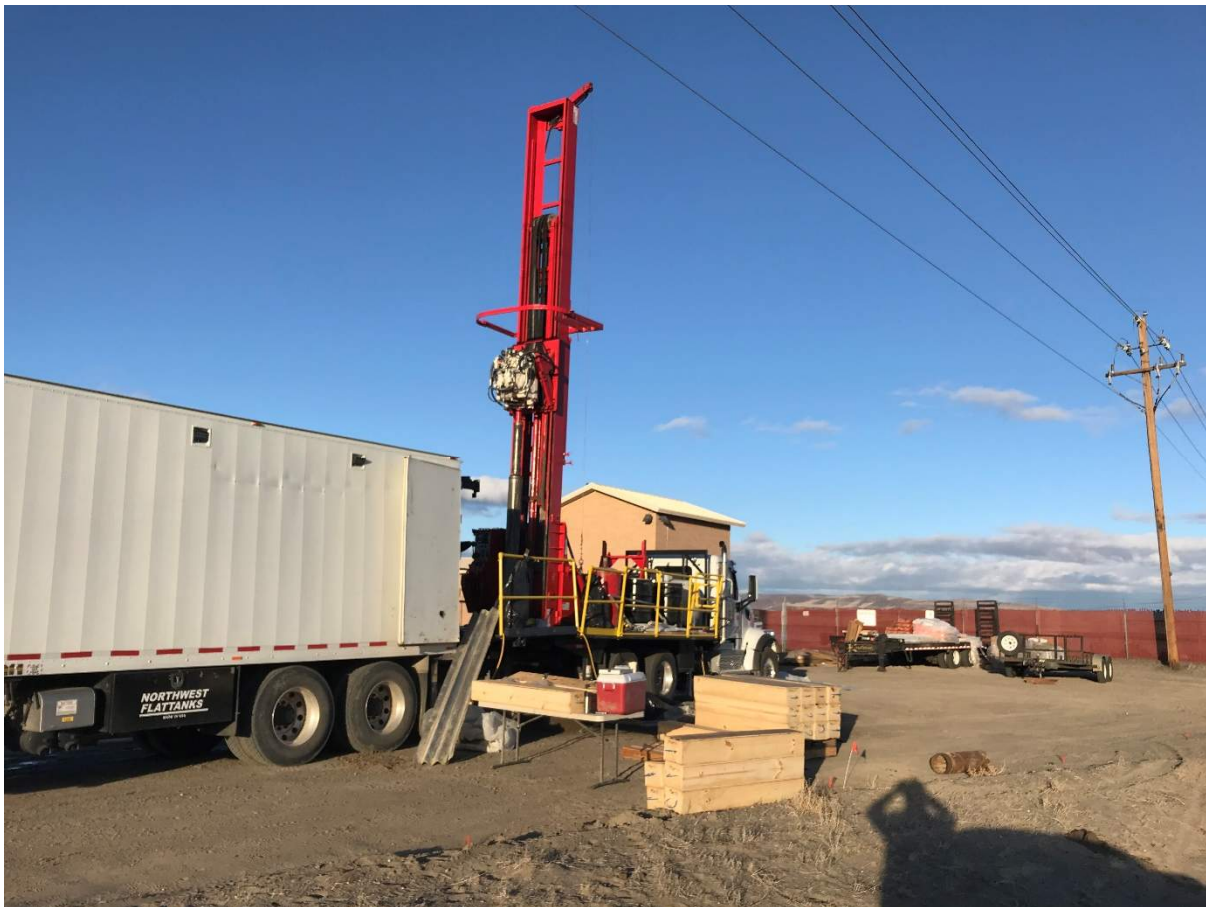
Figure 6. Photo of sonic drill rig and support vehicles
